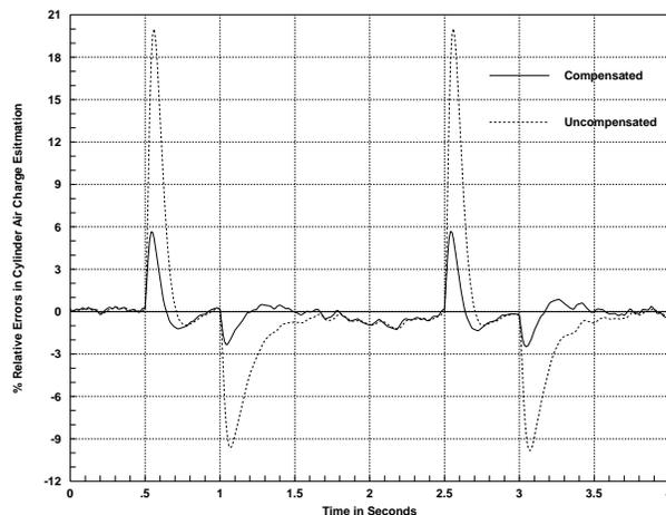
Figure 2: Percent relative errors in air charge estimation.
