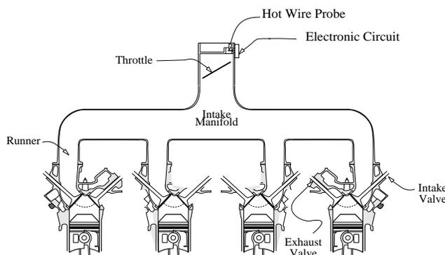
Figure 1: Schematic of air path in engine.
