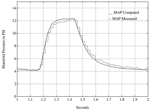
Figure 5: Comparison of measured and computed manifold pressure.
