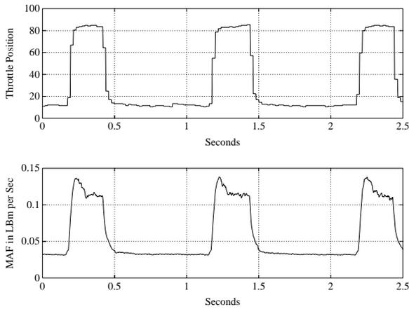
Figure 4: Engine operating conditions at nominal 1500 RPM.
